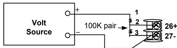
**Figure 5-6 Wiring Connections for 0 to 10 Volts**
