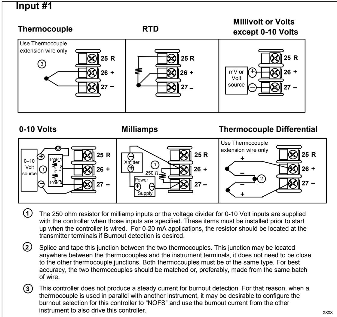
**Figure 2-6 Input 1 Connections**
