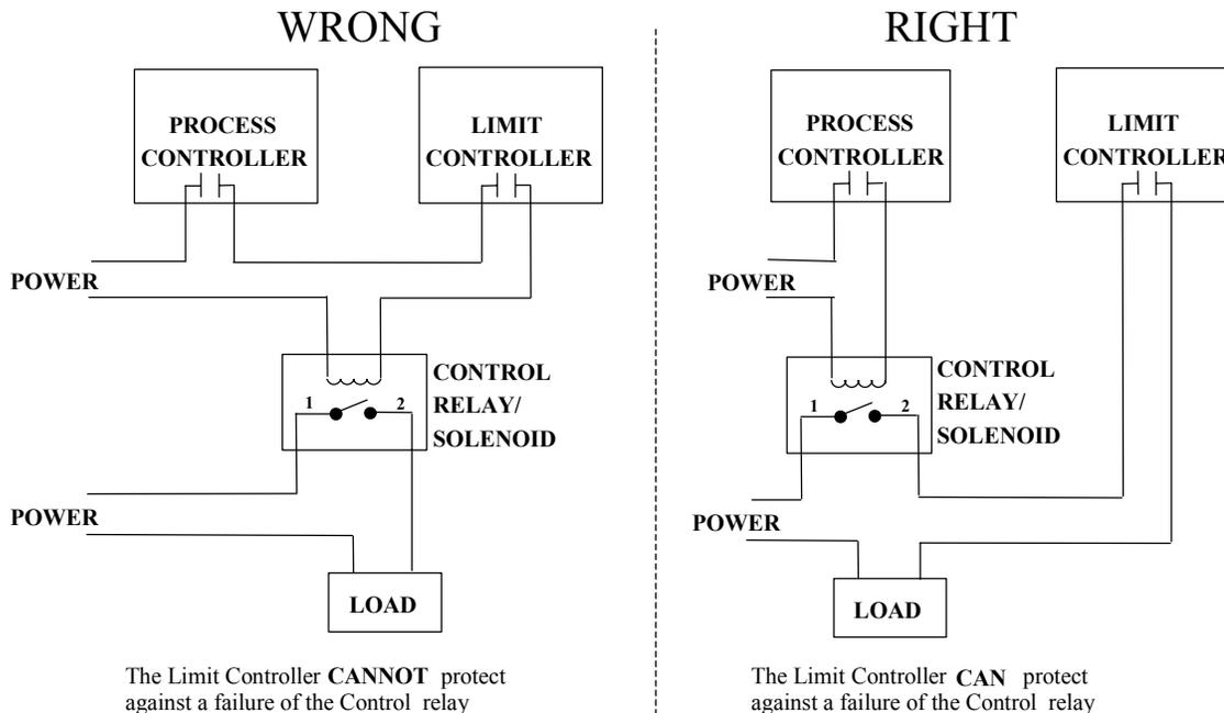
**Figure 2-15 Limit Controller Application Diagram**
