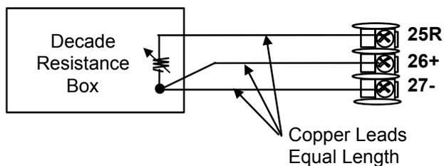
**Figure 5-4 Wiring Connections for RTD (Resistance Thermometer Device)**
