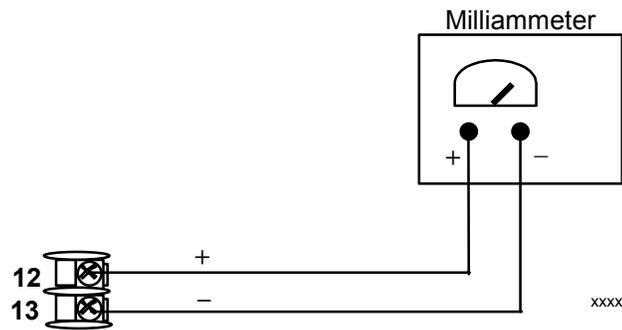
**Figure 6-1 Wiring Connections for Calibrating Auxiliary Output**
