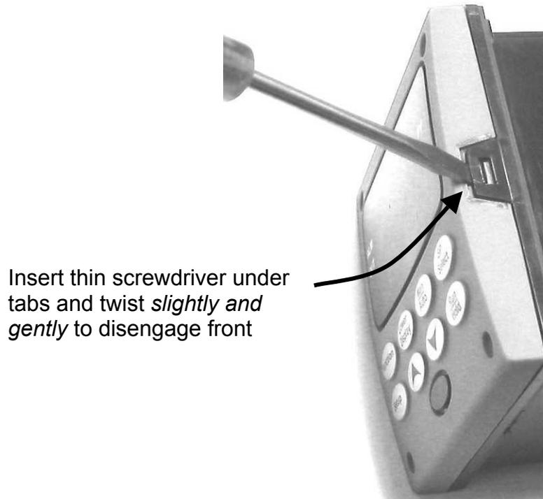
Using a thin screwdriver, *gently* twist the screwdriver to pry the side tabs from the front face. Pry just enough to release it, *otherwise you'll bend or break the tab*. If you break or bend the tab and can't reattach the front snugly, you'll need to reattach the front using the 4 NEMA4 screws provided. See Figure 2-3 on page 17.
