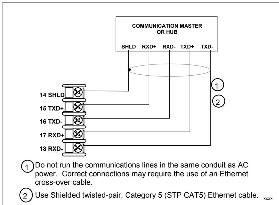
**Figure 2-11 Ethernet Communications Option Connections**
