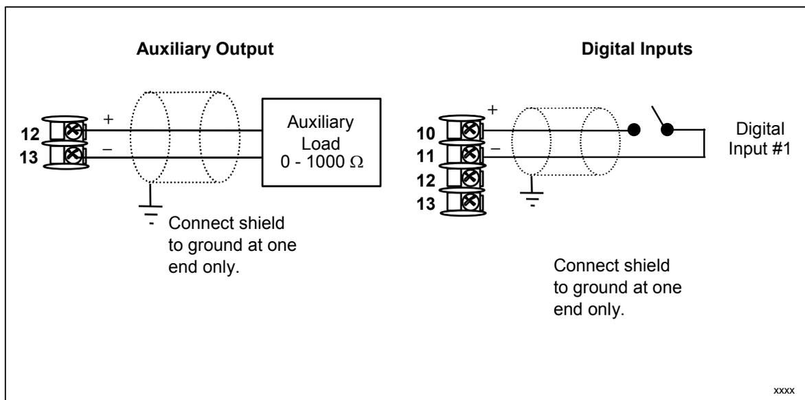
**Figure 2-12 Auxiliary Output and Digital Inputs Option Connections**
